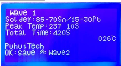
**STEP 2** After selecting curve, press OK/RETURN Button to return to the main menu. Select "Execute Temp Curve", then press OK/RETURN Button to execute.
