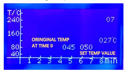
**STEP 3** Press OK/RETURN Button to set the temperature value, and then the system will automatically jump to the next time point. Each time point interval is 5 second.
