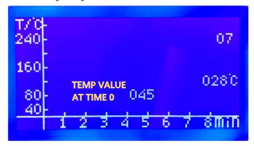
**STEP 2** Press ▲/▼ Button to change the temperature value at current time.
