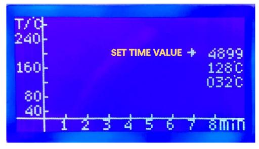
**Step 5** After setting the time value, press OK/RETURN Button to execute the thermostatic control function. When the work done, the machine will stop automatically (the machine will beep when the process stops)
